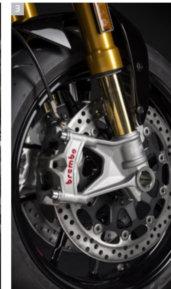
3 Radially mounted Brembo Stylema® monobloc 4-piston callipers
